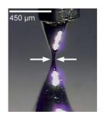
A great Galn: Micrometer-sized conformal electrodes formed from the title compound are shown to be ideal for measuring the electrical properties of self-assembled monolayers. The image shows the bifurcation of the EGaln between a metal needle and an Ag surface (not shown) at the point indicated by the two white arrows. The portion above the arrows will form the EGaln electrode.
