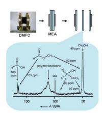
Methanol crossover and reaction intermediates are studied in a direct methanol fuel cell (DMFC) by means of <sup>2</sup>D and <sup>13</sup>C MAS NMR spectroscopy. A membrane electrode assembly (MEA) composed of three polymer electrolyte membrane (PEM) layers is used in the DMFC, and the middle PEM film is extracted to perform the NMR measurements (see image).
